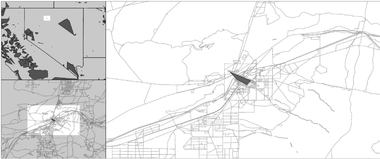
Fig. 8. Winnemucca volunteer fire department's estimated influence using census blocks. Note the polygon can be very finely matched by the blocks.
